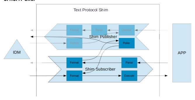
The poller uses the subscriber channel of the shim. It is an active component that interrogates the application. It adds one component.
